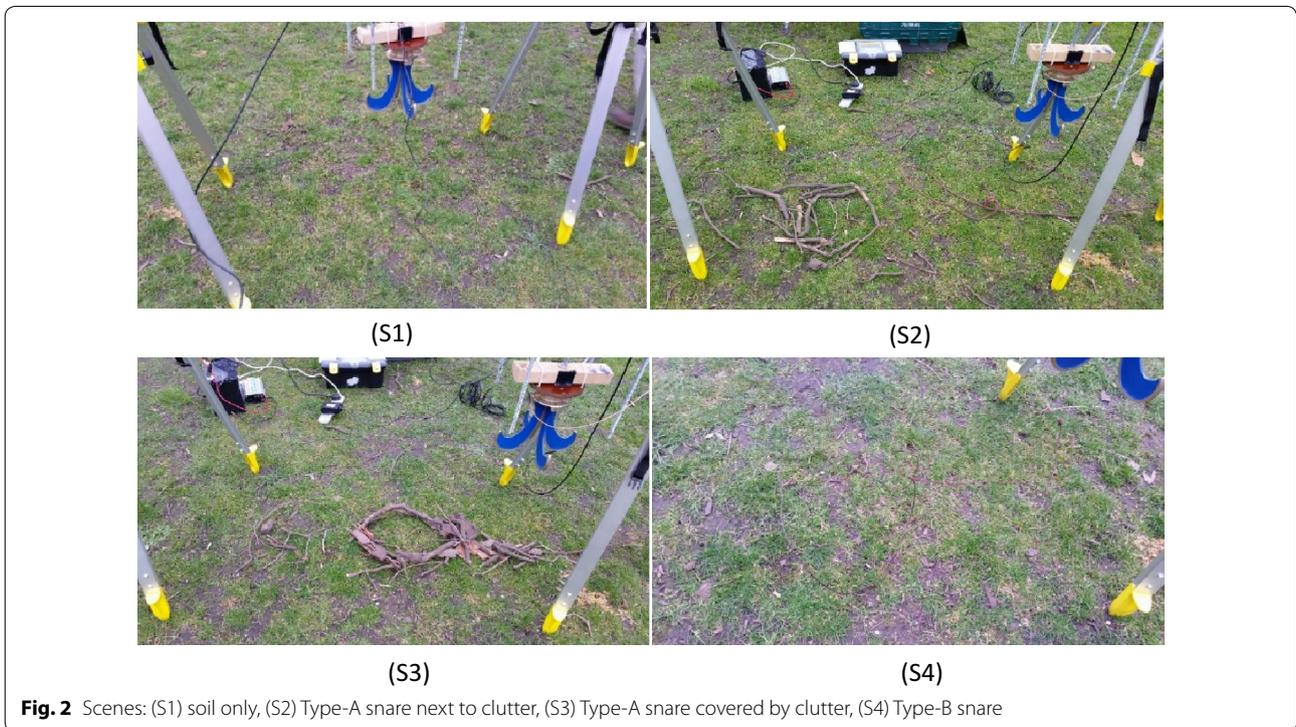
the following polarisations: horizontal polarisation (HH), and vertical polarisation (VV). The linear trajectory of the antenna allowed the illumination area to be progressively translated to create a two-dimensional scan known as a ‘B-scan.’ This technique is used to construct an image of the scene by integrating the 100 data points together (Daniels 2007).
