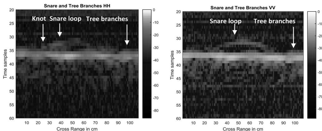
**Fig. 6** Scene 2—Type-A snare next to clutter—horizontal polarisation (left) and Vertical polarisation (right)
