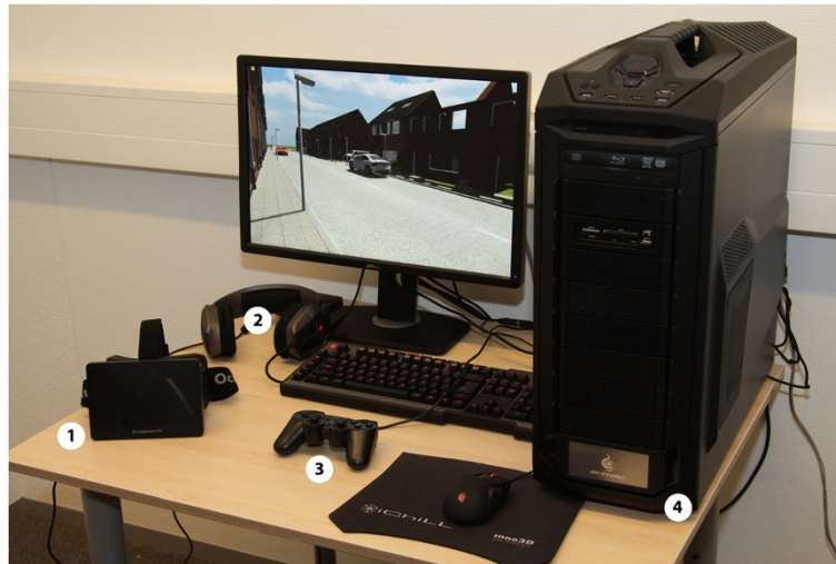
Figure 1 Virtual reality technology elements: 1) head-mounted display, 2) headphones, 3) controller, 4) (rendering) personal computer.
